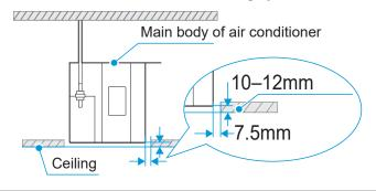
After adjusting the main body position and level, tighten the nuts on the mounting hook to secure the air conditioner in place.
