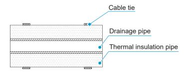
To prevent water from flowing back into the air conditioner when it stops running, the drainage pipe should be inclined downward to the outdoor side (drainage side), with a downward slope of 1/100 or more. The drainage pipe should be positioned in the same direction as the drainage outlet of the unit body in a left and right direction, so that the drainage pipe does not expand and collect water; otherwise, it may cause abnormal noise.
