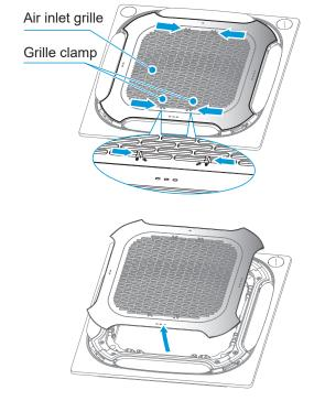
Remove the four fixing screws and remove the panel.
