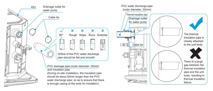
The drainage pipes of the unit (especially the indoor part) must be evenly wrapped with thermal insulation pipes and fastened with cable ties to prevent air from entering and producing condensate water.
