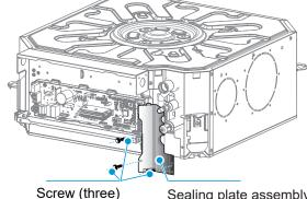
Screw (three) Sealing plate assembly
