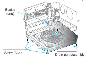
Remove the sealing plate assembly.
