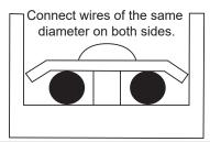
Do not press the power cables of the same wire diameter on the same side of the terminal. Do not use two power cables of different wire diameters for the same terminal blocks; otherwise, they can easily loosen due to uneven pressure and cause accidents, as shown in the figure below.
