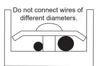
The connected power cable should be secured with a wire clamp to prevent loosening, as shown in the right figure.
