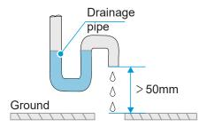
· Connection method of the drainage pipe:
